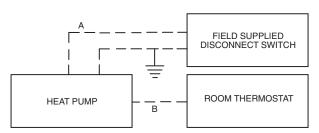
A = Two power wires for single-phase units.
